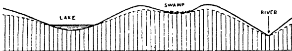
FIG. 23.—Diagram showing the Relation between Topography and Water-table in a Homogeneous, Permeable Rock.
